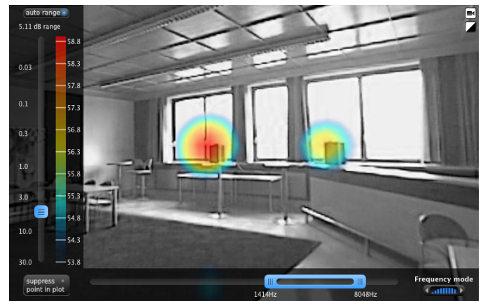
Fig. 13. Resolution of two loudspeakers with white noise output by using Nor848A-10 1.0m camera
