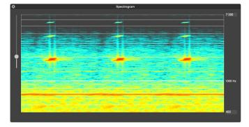
Lastly, due to the tonal nature of the noise it was possible to switch from the ordinary, robust wideband algorithm, to the adaptive algorithm for narrowband applications.
