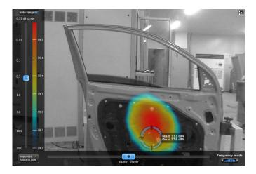
As opposed to the stationary sound from the electric engine, the high pitch squeak noise was only happening for a brief period of time, around 300 ms. By defining a scene in the sound level indicator pane of the acoustic camera software, it was then possible to analyse events happening only within the time frame of the extent of the scene. The scene is made by simply dragging the cursor over the region of interest in the software as seen below.
