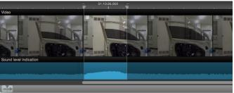
Now by calculating the average spectral density over that part of the recording, it was easy to see that in addition to the noise from the electric motor around 670 Hz, a high pitch tonal noise with a fundamental frequency around 1890 Hz could also be seen in the frequency spectrum. In addition harmonics of the fundamental frequency up to the 7th harmonic was visible in the spectrum.
