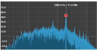
Now by filtering the frequency content of interest around the fundamental frequency, it was possible to get a clearer indication of the position of the source of the high pitch squeak noise as seen below.
