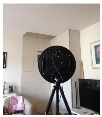
tions. The camera could be set up on the tripod, but also positioned on the floor, in a bed, on a couch or just hold it by hand all based on what part of the room one would like to listen to and get the acoustic image from. The 40 cm camera proved to be very handy in a measurement situation where it was not given beforehand exactly where the source of interest was positioned. In that way the camera could easily be used to scan around different parts of different rooms.
