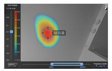
By using the virtual microphone, which enables the user to listen to a specific position in both real time and in a recording, one could clearly hear the sanitary noise from the recorded position at the roof. Also by enabling the bandpass filter one could further be able to filter out background noise and very clearly hear the sanitary noise from the piping. Based on these measurements one could deduct that the water pipes in were in fact not positioned as previously thought.
