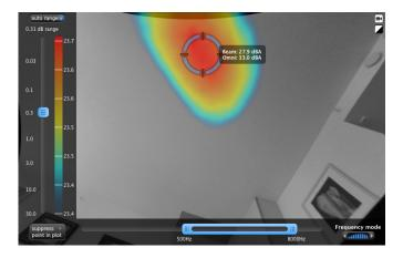
In addition to measurements in the living room subsecuent measurements were also made in the two bedrooms. These measurements displayed the same result, the energy of the noise did not come from the walls, but were confined to the roof. All in all this was a very strong indication that the problem was piping located in separating floors between apartments.
