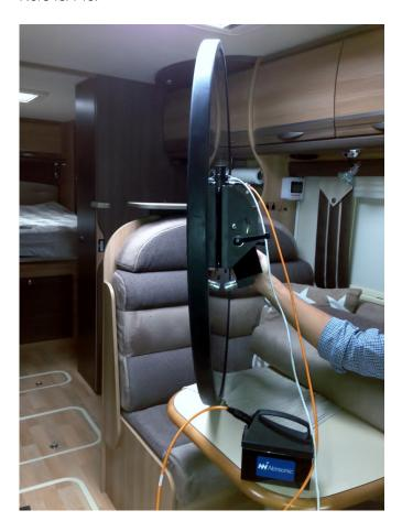
The measurements were done with one person driving the caravan, and another placing the camera dish on a table and performing the measurements. As the array dish itself weighs in at only 11 kg, it was easy to control it with one arm, and starting and stopping a measurement in the software on the MacBook with the other arm. No tripod was used or needed for the measurements.
