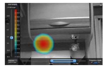
Finding the second noise source proved to be a trivial case after the fridge had already been ruled out as the source. Since most of the interior floor was wooden, is was thought that the creaking might originate from here, and this was the first position the camera was aimed at. Both coloring and listening with the virtual microphone confirmed this.
