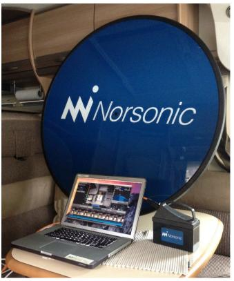
microphone to listen to the sound field from a specific direction. In addition it worked very well to enable the band pass filter when listening in order to filter out background noise such as engine noise and wheel noise.
