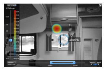
The position of the true source was seen more or less instantly to be inside a cabinet positioned on the wall of the car. This true source location was also confirmed when listening with the virtual microphone on a recording, and even when holding the ear into the cabinet when driving.
