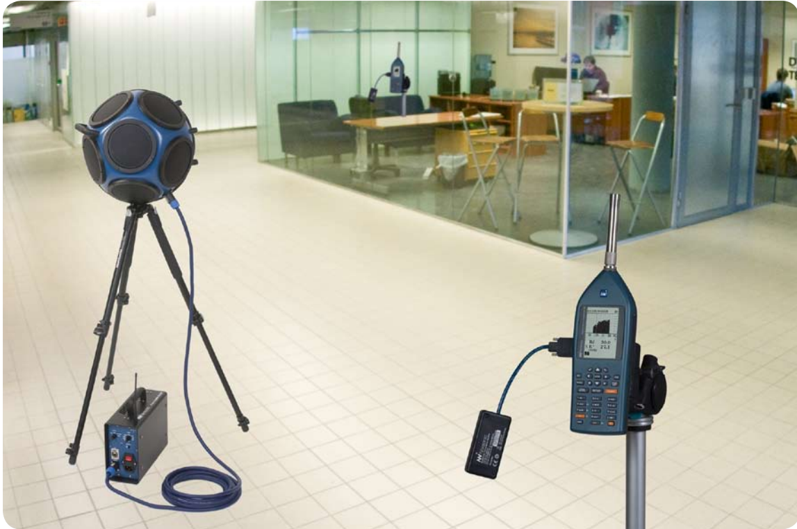
Dodecahedron Loudspeaker Nor276 and Power Amplifier Nor276 in situ with a Sound Analyser Nor140 fitted with wireless Bluetooth module for data transmission between sender and receivers room.
